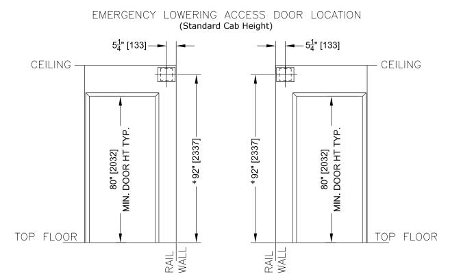
\* - 96" (2438 mm) TALL ELEVATOR CABS: THE VERTICAL DIMENSION IS 104" (2642 mm).
