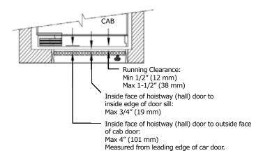
Upgrade Door Package Swinging Hall Door with Sliding Elevator Car Door
