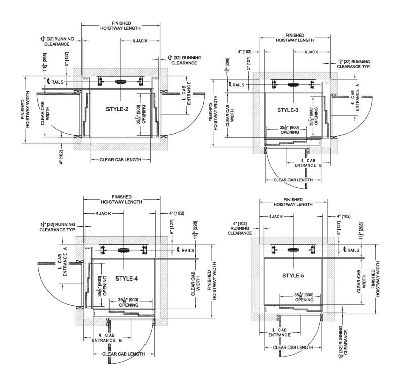
Premium Door Package - sliding elevator hall door with tandem sliding elevator car door
